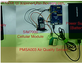
Fig. 4. Our air quality monitoring device developed with SAML11
